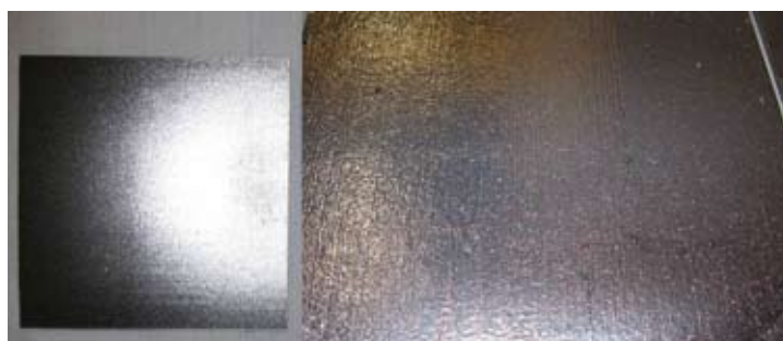
Figure 3. RGS wafers (156 mm x 156 mm), substrate side on the left, and free crystallising top surface on the right.
